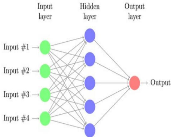
**Fig: Also called a Feedforward Neural Network (FFNN) Model with one hidden layer with 5 hidden units (since there is no backward connections between layers, viz., no loops).**
